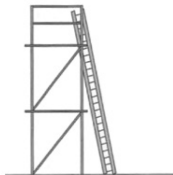
Extension ladder set against a scaffold
